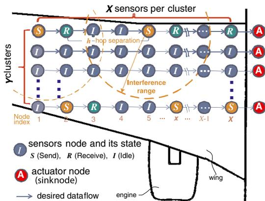
**Figure 1.** Wireless sensor/actuator network with a grid topology (hop separation  $h = 3$ ).
