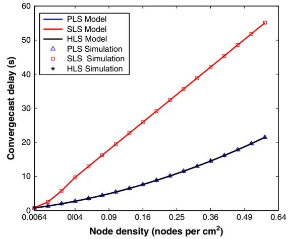
**Figure 9.** Total convergecast delay for SNR = 3.0 (equivalent  $h = 8$ ). PLS, parallel line scheduling; SLS, serial line scheduling; HLS, hybrid line scheduling.
