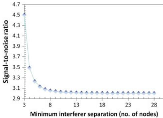
**Figure 6.** The required signal-to-noise ratio  $\epsilon$  versus minimum interferer separation  $h$  when  $\lambda = 3$ .
