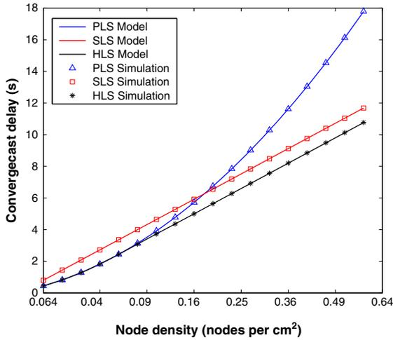
**Figure 7.** Total convergecast delay for SNR = 4.5 (equivalent  $h = 3$ ). PLS, parallel line scheduling; SLS, serial line scheduling; HLS, hybrid line scheduling.
