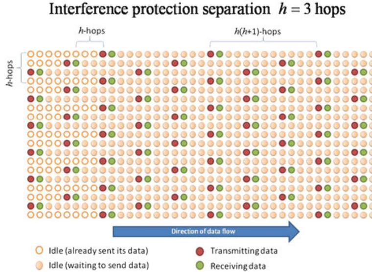
**Figure 5.** Illustration of hybrid line scheduling.
