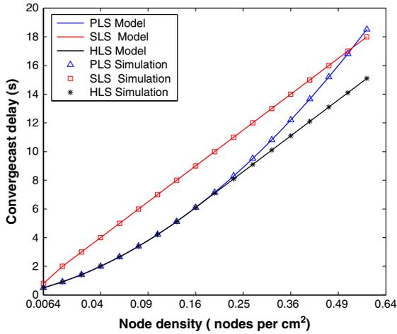
**Figure 8.** Total convergecast delay for SNR = 3.5 (equivalent  $h = 4$ ). PLS, parallel line scheduling; SLS, serial line scheduling; HLS, hybrid line scheduling.
